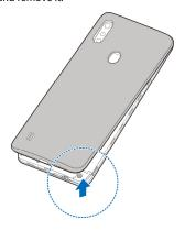
Hold the nano-SIM card with the cut corner oriented as shown and the microSDXC card with the metal contacts facing down and slide them into the card slots.
